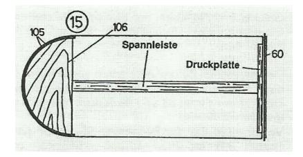
When dry, glue the two parts of the bulwark together and fasten them again until the glue is dry. Do not yet glue it to the deck!
